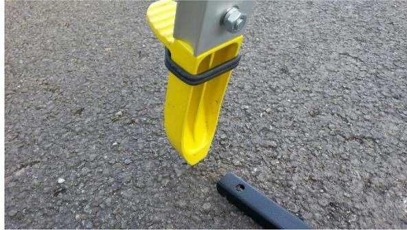
3. Finally, re-attach the star leg to elastic loop, repeat for each of the other two legs.
