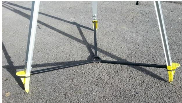
1. Position Tripod and Tripod Star in desired location with legs through the open elastic loops as shown.
