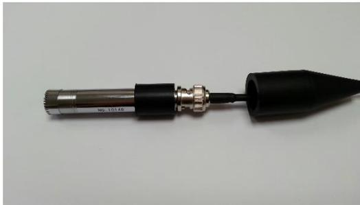
1. Connect the BNC plug from one end of the double booted cable to the microphone's BNC socket.
