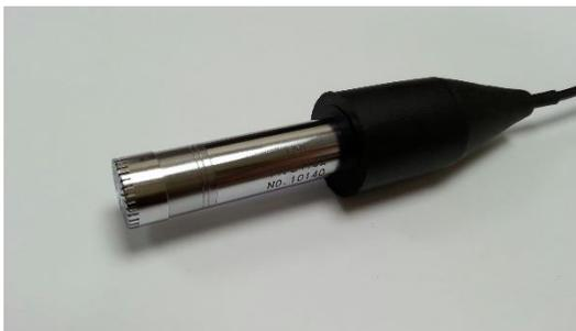
2. Next, ease the flexible rubber boot over the connector and rubber sleeve.
